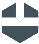
3 way join Three individual lightbars can be connected together to form t-shaped lighting fixtures.
